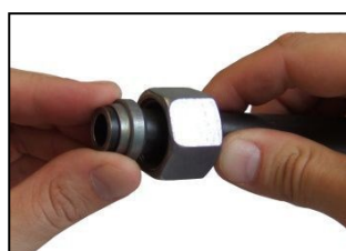
Position of cutting ring, union nut, tube
